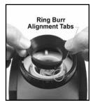
After replacing the burr, replace the silicone seal by lining up the two slots in the silicone seal with the small tabs on the top of the ring burr and slide the seal onto the ring burr.
