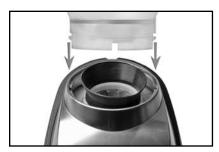
To replace the bean hopper, line up the two small tabs on the base of the hopper with their respective slots in the top of the grinder housing and insert the hopper into the grinder. Once the hopper is in place rotate it clockwise to your desired grind setting.
